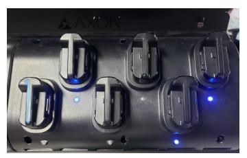
Image showing a TASER 7 Six-Bay Dock where LED indicator is blinking blue to show that a Log Sync Error occurred on the battery pack.
